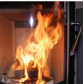
Light the fire and shut the door, leaving an open gap of approx. 10-15 mm.
