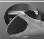
Remove the baffle plate and smoke chikane. Remove the blanking plate (3 M6 nuts) and its sealing.
