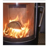
After approx. 5 min. - or when the flames are clear and stable - close the damper gradually.
